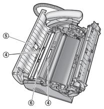
4 Clean the recording paper feeder roller (⑦) with a cloth moistened with isopropyl rubbing alcohol, and let all parts dry thoroughly.
